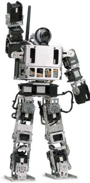
Figure 2.3: Mini-Hubo platform: 22 DOF, 46 cm tall miniature-size humanoid robot weighing 2.9 kg .
